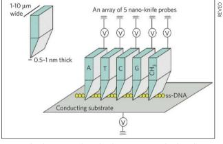
Reveo is developing a single-molecule sequencing technology that physically probes DNA.
