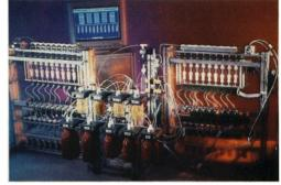
proach is array chemistry, a system involving dozens of parallel reactions for establishing structure/activity relationships. Glaxo Wellcome has developed proprietary parallel reactors, with efficient heating, cooling and stirring capability, and these are spreading rapidly throughout the labs. Automated, and therefore faster, purification equipment has also been developed. Automated HPLC means that large batches of compounds can be purified
