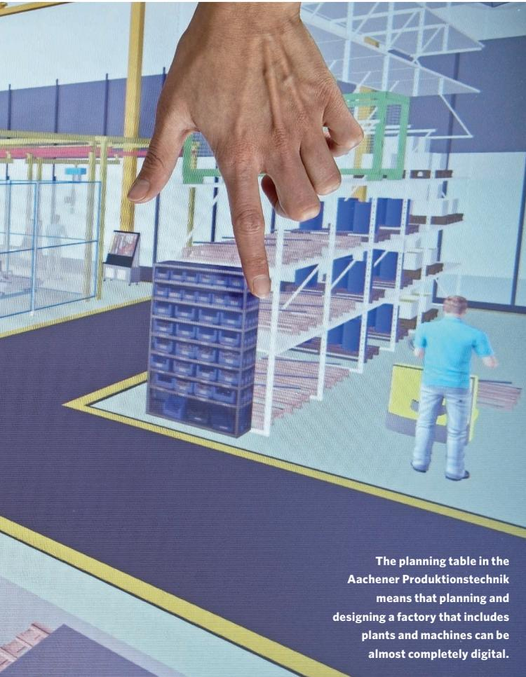
The planning table in the Aachener Produktionstechnik means that planning and designing a factory that includes plants and machines can be almost completely digital.
