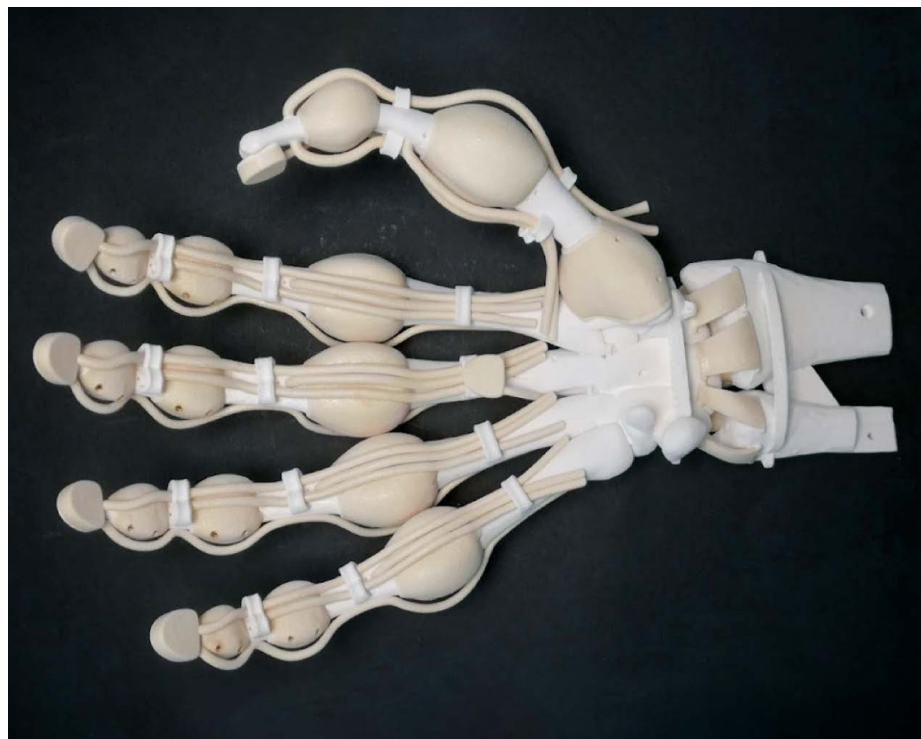
Figure 2 | A 3D-printed robotic hand. Buchner et al. 1 used their machine-vision-guided 3D printer to produce a robotic hand, which was printed using two different materials. The hand can be driven pneumatically to grasp objects in response to pressure applied at the fingertips.
