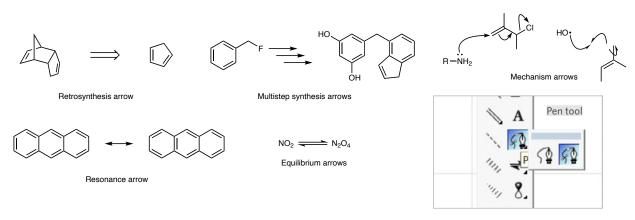
Ourly arrows in mechanism diagrams should be shown going from the centre of a breaking bond or lone electron pair to the centre of a forming bond or a specific atom. We recommend using the pen tool to position arrows accurately rather than using the template curved arrows in ChemDraw.
