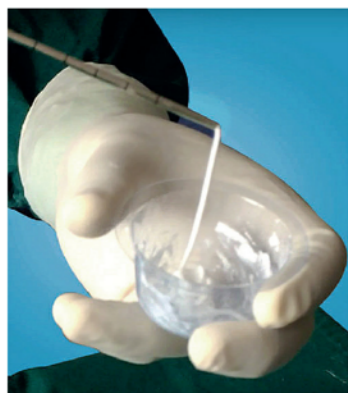
The calcium phosphate cement (CPC) material designed by Liu's team is biologically compatible and injectable.
