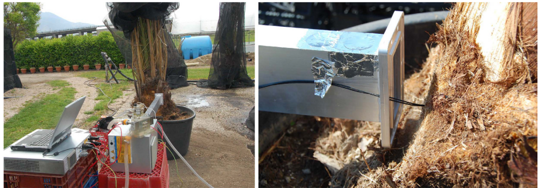
Figure 1. Experimental set-up to estimate the thermal parameters; (a) the palm is radiated by a WR340 waveguide connected to a microwave applicator; the incident power is measured by a circulator connected to a power meter; (b) the temperature in two points inside the palm is measured using an optical fiber thermometer.
