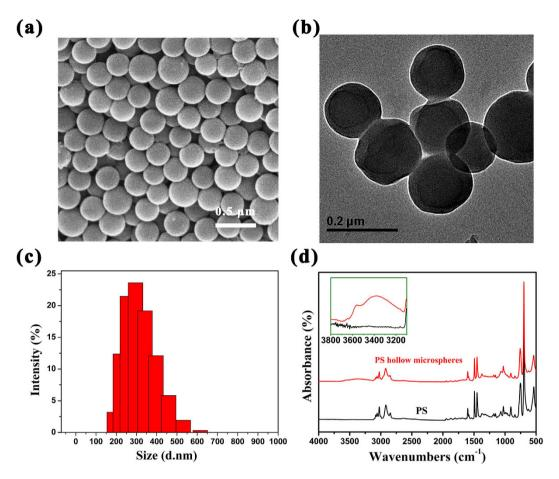
**Figure 1.** The structural properties of PS hollow microspheres measured by (a) SEM; (b) TEM; (c) Diameter distribution and zeta potential; (d) FT-IR spectroscopy. The ratio of styrene to deionized water was 5% in reaction system.
