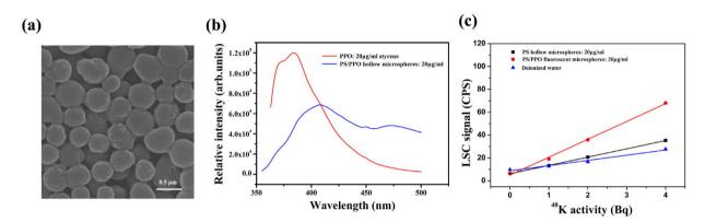
**Figure 6.** (a) The SEM analysis of raspberry-shape morphology for PS/PPO microspheres. (b) The emission spectrum of PPO and PS/PPO microspheres. (c) The LSC signal of  $^{40}$ K (14.4 Bq/g) measured by liquid scntillation counter with PS hollow microspheres, PS/PPO microspheres and water solution, where the measured time was 5 minutes.
