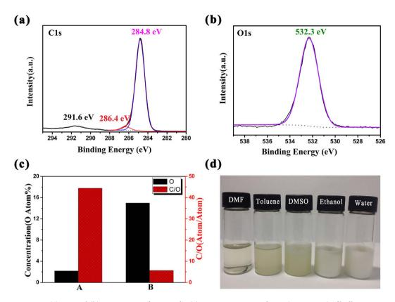
**Figure 2.** (a) C1s and (b) O1s spectra of XPS study; (c) Oxygen content and C/O (atom/atom) of hollow microspheres by using XPS spectroscopy and SEM-EDS element analysis; (d) The dispersibility of PS hollow microspheres in water, ethanol, DMSO, DMF and Toluene solution, respectively. The reaction condition was the same as Fig. 1.
