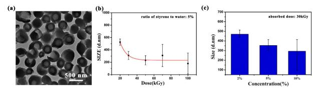
**Figure 5. PS hollow microspheres prepared by different reaction condition.** (a) TEM analysis of PS hollow microspheres prepared in the presence of oxygen; (b) The size of microspheres with different absorbed dose and (c) different concentration ratio of monomer to water. The reaction condition was the same as Fig. 1.
