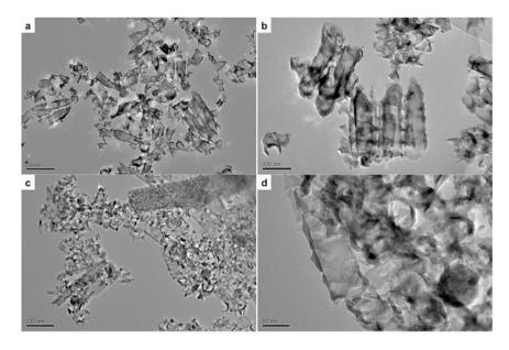
**Figure 2. TEM micrographs of TiO<sub>2</sub> nanotubes. (a)** Low magnification and (b) high magnification images of ethylene glycol (organic) electrolyte fabricated TiO<sub>2</sub> nanotubes. (c) Low magnification and (d) high magnification images of HF/H<sub>2</sub>O (aqueous) electrolyte fabricated TiO<sub>2</sub> nanotubes.
