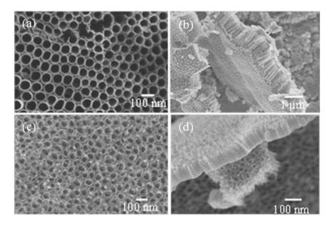
Figure 1. SEM images of TiO<sub>2</sub> nanotube array films separated from substrates. (a) Top and (b) lateral views of the nanotubes fabricated using the EG/NH<sub>4</sub>F electrolyte. (c) and (d) show the images of the corresponding regions in films grown in the water/HF electrolyte.
