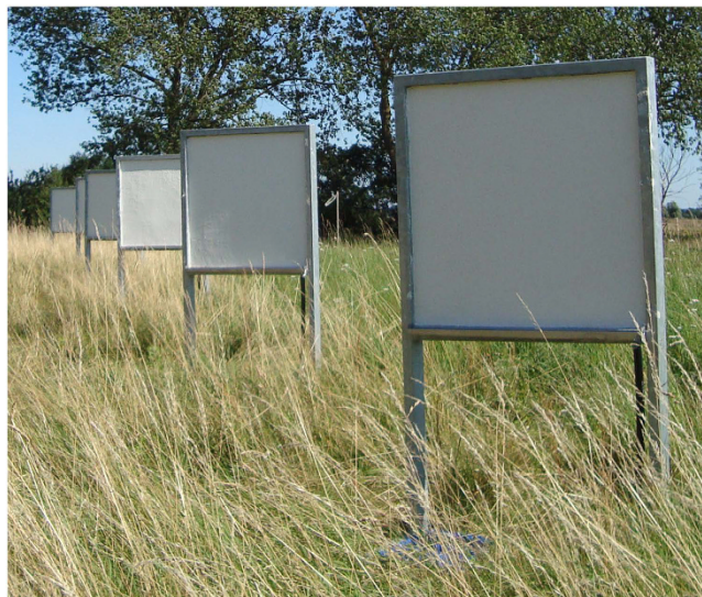
Figure 1. Experimental setup: artificial walls (1 × 1 m) for field emissions.
