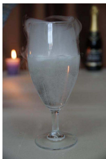
Figure 5. (a) Photo of hydrate decomposition in warm water. (b) Dynamics of degassing of hydrate sample produced in the experiment during the decomposition (solid line); dynamics of decomposition of the same amount of ice (dashed line): m –mass of the sample during decomposition; m_0 –initial mass of the sample; k –mass fraction of the gas in the hydrate.
