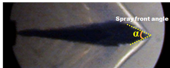
Figure 6. Illustration of spray front angle.
