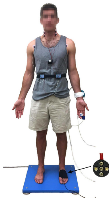
Figure 1. Data collection for comparing weighing scale-based pulse transit time (PTT) to conventional pulse arrival time (PAT) as markers of blood pressure (BP) in humans. (A) Ballistocardiography (BCG) and foot photoplethysmography (PPG) waveforms were measured with a custom system similar to a weighing scale; ECG, finger PPG, and impedance cardiography (ICG) waveforms were measured with standard sensors; and a reference finger cuff BP waveform was measured with a volume-clamp device. (B) The waveforms were recorded during three baseline periods (R1, R2, R3) and three interventions (mental arithmetic (MA), cold pressor (CP), post-exercise (PE)) to increase BP but change the pre-ejection period (PEP) differently.
