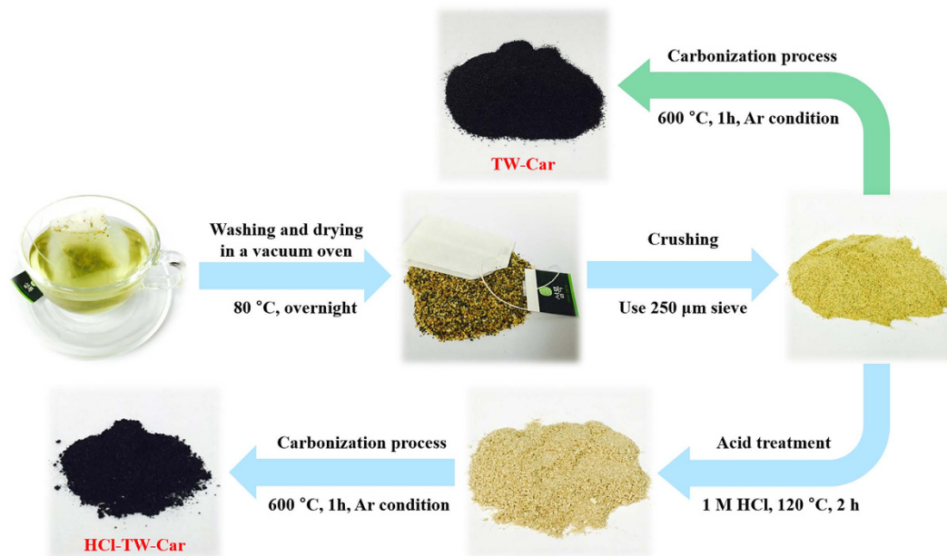
Figure 1. Synthesis process with/without acid treatment for the production of porous carbon derived from tea waste.
