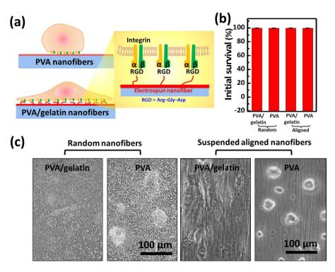
**Figure 3. PVA and PVA-gelatin nanofibers and cell growth.** (a) Schematics of cell attachment on PVA and PVA-gelatin nanofibers (b) Initial survival of cells after seeding on the nanofibers for 24 h. (c) cell morphology of growing cell on the PVA and PVA-gelatin random and aligned fibers.
