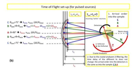
**Figure 3. Instrument layout.** (a) The layout for the CW instrument-concept suitable for continuous sources; and (b) the layout for the TOF instrument-concept suitable for pulsed sources. The different colours represent different wavelengths, which also have different energy resolutions, different velocities and, in turn, different TOF.
