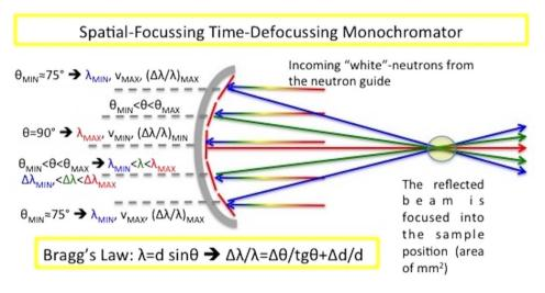
**Figure 2.** The primary spectrometer concept. The different colours represent different wavelength, which also have different energy resolutions.
