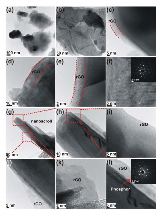
**Figure 2.** (**a**–**f**) TEM and HRTEM images of GO 1200, (**g**–**l**) TEM and HRTEM images of GO 1350. The wrapping of rGO over GO 1200 phopshors is clearly visibile, while in GO 1350, the self-wrapping of rGO sheets results in the formation of nanoscrolls.
