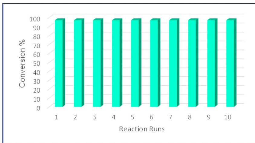
Figure 3. Investigation of the catalysis performance in 10 runs. (Reaction conditions: 0.1 M PhI and 0.25 M K_2CO_3 in MeOH:H 2 O 3:1, 0.3 mL.min -1 , 5% Pd/C; 2 h each reaction run).
