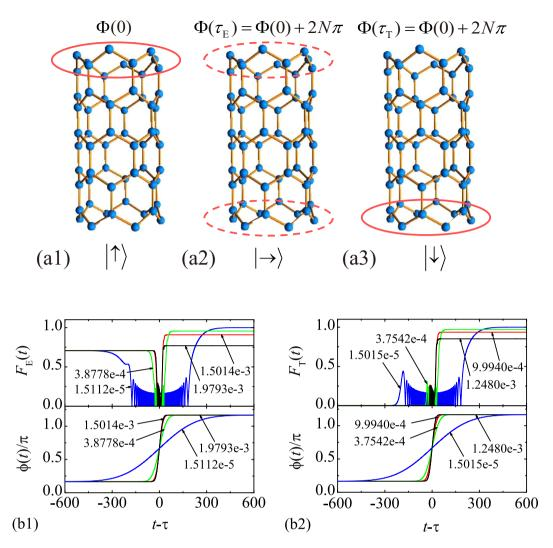
Figure 4. Schematic illustration of the manipulation for a perfect edge state in a graphene tube, which is represented by a red circle. When varying the flux slowly, state (a1) can evolve to (a2) and (a3), where (a2) represents a maximal entangled state. (b1) and (b2) are plots of the fidelities under the control of Gaussian pulse fluxes with several typical  $\sigma$ . Here the time t is in units of  $1/\Delta$ .
