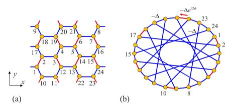
**Figure 6.** (a) Sketch of a graphene tube with periodic boundary condition for N = 3, M = 8. The lattice is indexed in another way. (b) Based on this method, the original lattice can be regarded as an 24-site ring with long-range hoppings.
