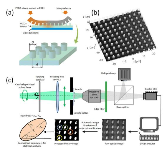
**Figure 1.** Sample and experimental setup. (a) Sketch of the soft lithography method for micro-pillar fabrication on glass substrate (pillar diameter  $D = 3 \mu m$ , period  $\Lambda = 5 \mu m$ , height  $h = 1.5 \mu m$ ); (b) 3D representation of an AFM topography map of the micro-pillar array; (c) sketch of the optical setup, the data acquisition and the processing flow.
