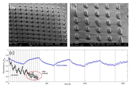
**Figure 3. Stability of pillar deformation cycles.** Exemplary SEM pictures of individual all-PAZO pillars: (**a**) before and (**b**) after a laser exposure with linear polarization (irradiation time 400 s). (**c**) Time-resolved mean roundness values for pillars during laser irradiation with time-varying polarization states (black circles: PAZO pillars, blue circles: PAZO+PMMA pillars).
