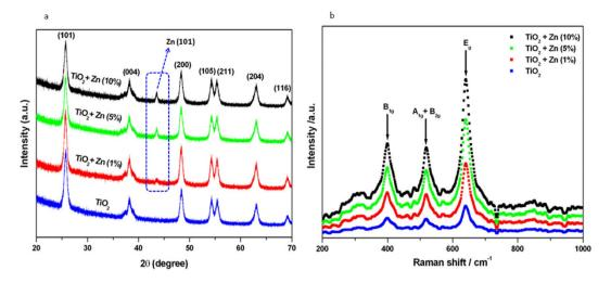
**Figure 2.** XRD and Raman characterization of pure and Zn-doped TiO<sub>2</sub> NPs. (a) XRD spectra and (b) Raman spectra.
