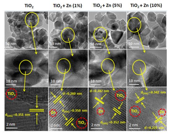
**Figure 1. Transmission electron microscopy characterization of pure and Zn-doped TiO**<sub>2</sub> **NPs.** Upper & middle panels represent the low resolution images while lower panel shows the high resolution images.
