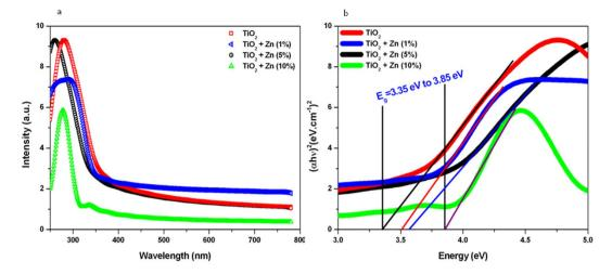
**Figure 3.** Optical characterization of pure and Zn-doped TiO<sub>2</sub> NPs. (a) UV-visible absorption spectra and (b)  $(\alpha h \nu)^2$  vs photon energy plots of the corresponding sample used to determine their band gap energy levels.
