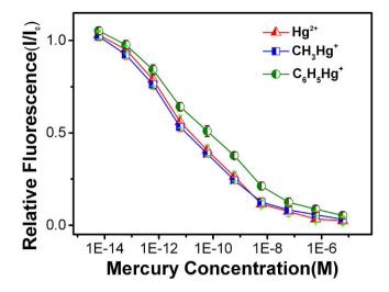
Figure 4. Normalized fluorescence intensity variation (I/I<sub>0</sub>) of R6G/MPA-NPG as a function of mercury ion (Hg<sup>2+</sup>, CH<sub>3</sub>Hg<sup>+</sup> and C<sub>6</sub>H<sub>5</sub>Hg<sup>+</sup>) concentration.
