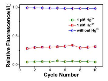
**Figure 5.** Recyclability test of the R6G/MPA-NPG sensor. Normalized fluorescence peak intensities with 1 nM (square dots) or  $1 \mu$ M (round dots) Hg<sup>2+</sup> in the aqueous solution for 10 cycles. I<sub>0</sub> indicates the fluorescence intensity of the R6G/MPA-NPG sensor before the recyclability test.
