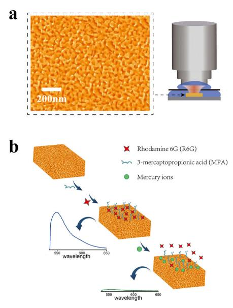
**Figure 1.** Characterization of the R6G/MPA-NPG fluorescence sensor. (a) Typical SEM micrograph of NPG and the experimental set-up for the Hg<sup>2+</sup> detection. (b) Schematic representation of the preparation of the R6G/MPA-NPG fluorescence sensor for detection of mercury ions based on displacement of R6G units on NPG.
