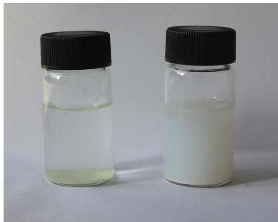
Figure 8. Photographs of the dispersions of bulk g\text{-C}_3\text{N}_4 (left) and TECN (right) in water, after sonication for 10 min and storage for 6 h under ambient conditions.
