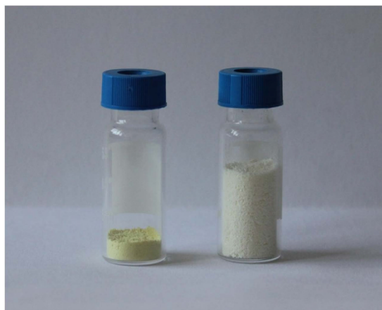
Figure 3. The volume comparison of 100 mg powder of bulk g\text{-C}_3\text{N}_4 (left) and TECN (right).
