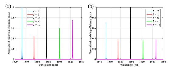
**Figure 6.** Receiving spectrum of the composited device shown in Fig. 5(a) when the GeSe is in (a) amorphous state and (b) crystal state, respectively.
