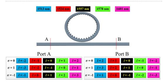
Figure 4. Comparison of resonant wavelengths for vortex beam with different SAMs and TCs based on the detection from Port A and Port B.
