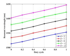
Figure 7. Resonant wavelength of different OAM states versus duty cycle of the GeSe gratings.
