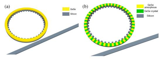
**Figure 5.** Diagram of the composite OAM receiver that has a (a) GeSe annular film and (b) GeSe gratings consist of alternate states on top of the resonator as the cladding layer. The duty cycle of the gratings is 0.5.
