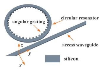
**Figure 1. Diagram of the proposed OAM receiver.** The circular resonator with angular gratings patterned along the inner wall couples the normally incident azimuthally polarized vortex beam to an access waveguide.
