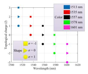
Figure 3. Resonant wavelengths for vortex beam with different SAMs.
