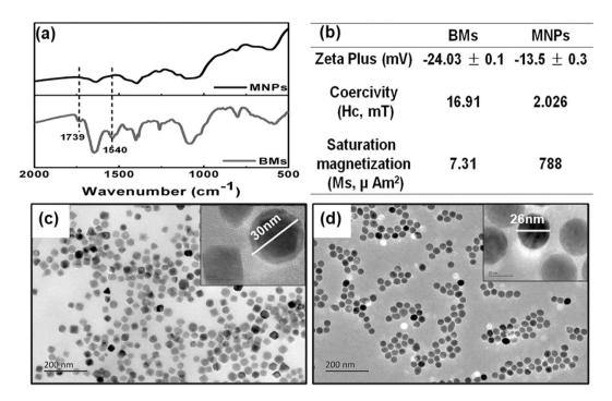
**Figure 1.** Characterization of the BMs and MNPs. (a) FTIR spectra of BMs and MNPs. (b) Zeta Plus and magnetic hysteresis values of the BMs and MNPs. (c,d) HRTEM images of the BMs (c) and MNPs (d).
