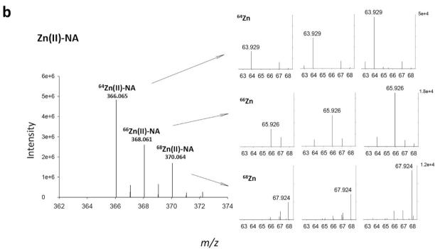
**Figure 2. Spectra of the free Zn released from Zn(II)-DMA/NA complexes.** The release of free Zn isotopes (right panels) from the corresponding Zn-complexes was obtained in positive ESI mode with Orbitrap-MS at fragmentation energy HCD 120, 130 and 150%.
