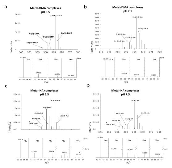
Figure 4. Identification of metal-DMA and metal-NA complexes under physiological pH conditions. The metal complex mixtures were prepared in pH 5.5 (a,c) and pH 7.5 (b,d) and identified with the released free metals (lower panel) in positive ESI mode with Obritrap-MS. The spectra of the released free metals were obtained in ESI-MS/MS with fragmentation energies HCD-90%. Asterisk denotes the ferric ion.
