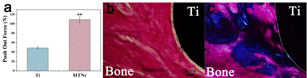
Figure 5. Analysis of newly formed bone on the surface of cylindrical rods modified with nanorods with a medium density. (a) Push out forces of Ti and MTNrs after implanted into rabbit 12 weeks. This data is reported as the mean \pm standard deviation. **p < 0.01 compared with the pure Ti surface. (b,c) Masson staining of the sections of implants showing MTNrs (c) can efficiently induce the formation of new bone tissue in comparison with pure Ti (b).
