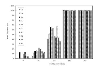
Figure 5. Effect of shaking speed on metal recovery from a  $4 \text{ cm} \times 4 \text{ cm}$  PCB piece after 22h at room temperature.
