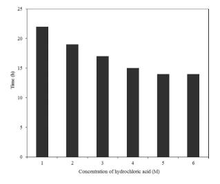
Figure 4. Effect of HCl concentration on the time required for complete metal recovery from a  $4 \text{ cm} \times 4 \text{ cm}$  PCB piece at 150 rpm and room temperature.
