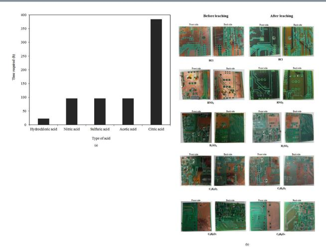
Figure 2. Effect of various lixiviants on (a) the time required for metal recovery from the PCB pieces and (b) the surface appearance of the PCB pieces before and after leaching.
