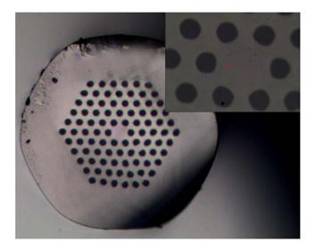
Figure 2. Cross section of the end face of fiber made from silicate glass under different magnification.
