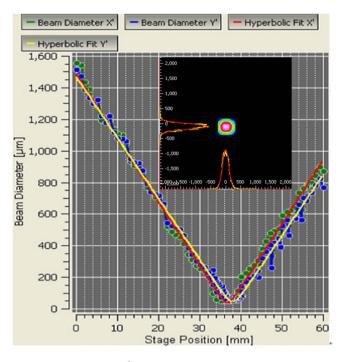
Figure 4. Measured  $M^2$  factor at an output power of 0.8 W; Inset shows mode field distribution of the fiber.
