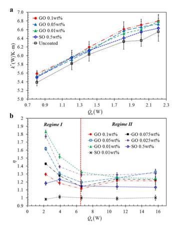
**Figure 5.** (a) Thermal conductance of uncharged TPCTs coated with thin GO and SO nanoparticles depositions as a function of  $\dot{Q}_{\rm a}$  during the heat conduction experiments. (b) The evaporator heat transfer coefficient augmentation ratio,  $\eta$ , as a function of  $\dot{Q}_{\rm a}$  with nanoparticles weight ratio as a parameter. Two distinct regimes –  $\dot{Q}_{\rm a}$  < 6.5W and  $\dot{Q}_{\rm a}$  > 6.5W can be clearly identified.
