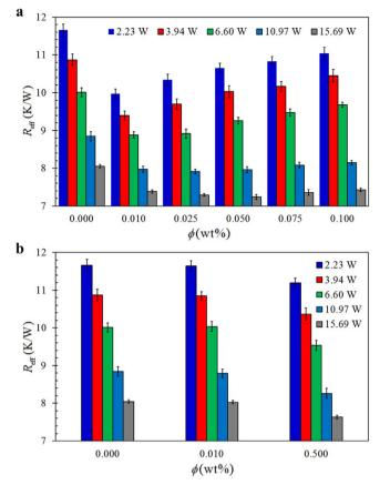
Figure 4. Effective thermal resistance,  $R_{\text{eff}}$  as a function of nanoparticles weight ratio,  $\phi$ , of (a) GO nanofluids, and (b) SO nanofluids, charged TPCTs at different  $\dot{Q}_{a}$ .
