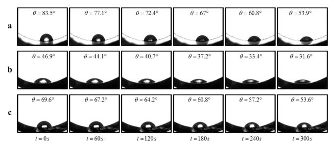
Figure 6. Time-lapse images of a  $2\mu l$  water droplet residing on (a) 0.1 wt% GO deposited layer, (b) 0.5 wt% SO deposited layer, and (c) uncoated glass surface, over a time span of 5 minutes. For each 60-s interval, the corresponding contact angle is recorded and depicted.
