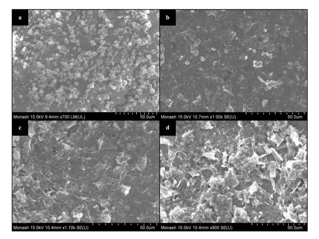
**Figure 8. FESEM images of SO nanoparticles and GO sheets deposited on the glass surface of the evaporator section of TPCT:** (a) 0.5 wt% SO nanoparticles, (b) 0.01 wt% GO sheets, (c) 0.05 wt% GO sheets and (d) 0.1 wt% GO sheets. The well distributed, closely-packed layered structure of GO sheets can be easily distinguished from the disorderly distributed spherical SO nanoparticles deposition. Higher concentration of GO sheets deposition is manifested in thicker strands.
