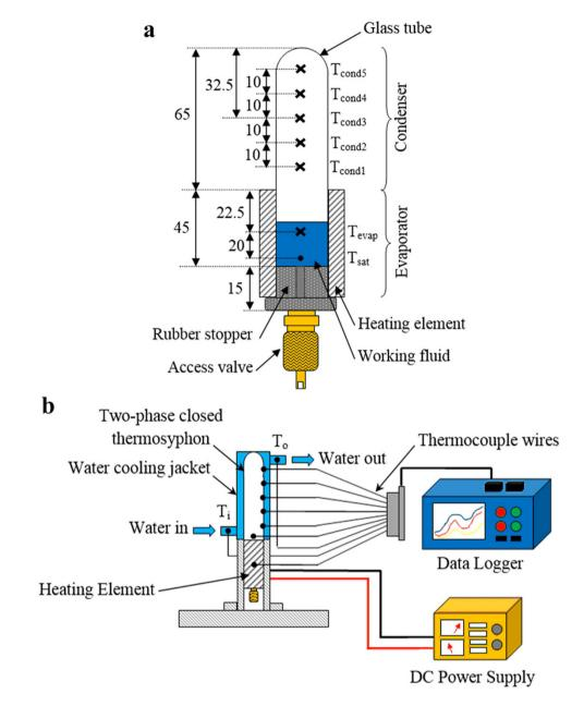
**Figure 1.** (a) Schematic diagram of a TPCT with temperature measurement points. (b) The experimental setup for the evaluation of performance of nanofluid charged TPCT.
