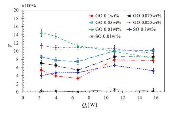
Figure 3. Variations of  $\Delta T$  reduction ratio,  $\psi = (\Delta T_{\rm nf} - \Delta T_{\rm o})/\Delta T_{\rm nf}$ , of GO and SO nanofluids charged TPCTs as a function of  $\dot{Q}_{\rm a}$ , with the nanofluid concentration being a parameter.
