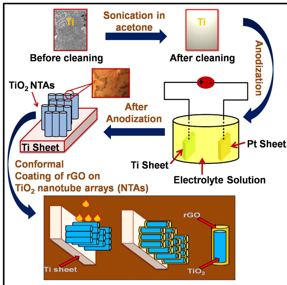
Figure 1. The synthesis process for highly oriented architecture of \text{TiO}_2 NTAs via anodization technique with conformal coating of rGO on highly oriented annealed \text{TiO}_2 3D NTAs samples (40 V, 4 hours, 500^\circ\text{C} ).
