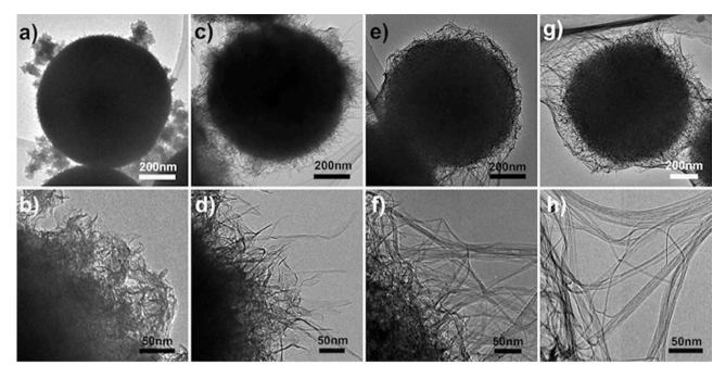
Figure 2. TEM images of sodium titanates samples collected after hydrothermal reactions for different durations. (a, b) 15 min, (c, d) 1 h, (e, f) 12 h, and (g, h) 48 h.
