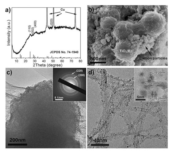
Figure 5. (a) XRD pattern, (b) SEM image, (c) TEM micrograph, SAED pattern (inset), (d) high-magnification TEM and HRTEM (inset) of the  $TiO_2$ -B material after discharge-charge measurements at 10 C for 1000 cycles.
