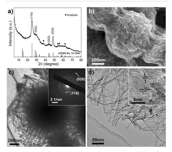
Figure 3. (a) XRD pattern, (b) SEM image, (c) TEM micrograph, SAED pattern (inset), (d) high-magnification TEM and HRTEM (inset) of the as-prepared porous  $TiO_2$ -B spheres constructed by nanotubes.
