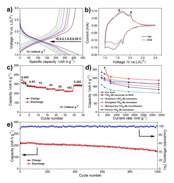
**Figure 4. Electrochemical properties of the TiO**<sub>2</sub>**-B material.** (a) galvanostatic discharge-charge curves at different current rates; (b) the first two CV curves at a sweep rate of  $0.2 \text{ mV s}^{-1}$ ; (c) rate performance; (d) comparison of rate capability between this work and other previously reported works at various current densities; (e) cycling performance at high current rate of 10 C over 1000 cycles.
