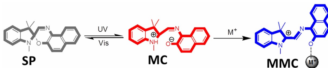
Figure 2 | The interconverts of spirooxazine among the closed form, merocyanine (MC) form and metallic merocyanine (MMC) form.
