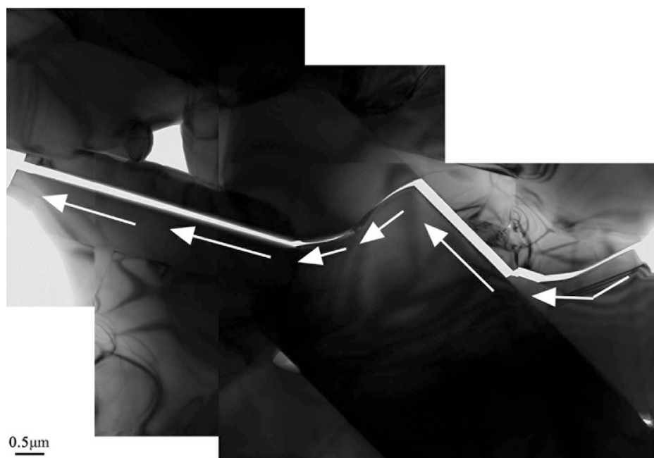
Figure 10 | A TEM image showing crack propagation in the fired composite.
