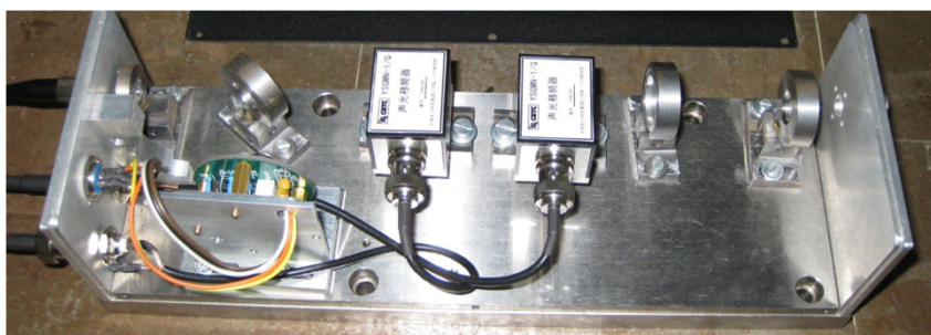
Figure 5 | Laser feedback interferometer based on external frequency-shifted feedback.
