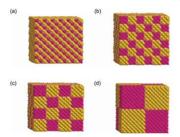
Figure 1 | The structures of the isotopic nanoscale 3D phononic crystals three dimensional periodic arrangements of <sup>28</sup>Si and <sup>M</sup>Si atoms. From (a) to (d), the period lengths of those 3D phononic crystals are 2, 4, 6 and 12 units, respectively. The lattice constant is 0.543 nm, that is, 1 unit represents 0.543 nm. In simulations, the periodic boundary condition is applied in all three directions.
