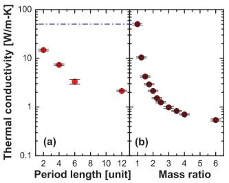
Figure 3 | (a) Thermal conductivity versus the period length of isotopic nanoscale 3D phononic crystal of Si. The mass ratio is 2. The dash dot line corresponds to the molecular dynamic result of thermal conductivity of pure <sup>28</sup>Si. (b) Thermal conductivity versus the mass ratio of isotopic nanoscale 3D phononic crystals of Si. The period length is 12 units. All values are calculated at 1000 K.
