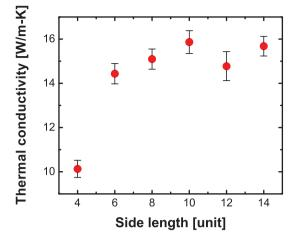
Figure 2 | Thermal conductivity versus the side length of simulation cell. The mass ratio of the 3D isotopic phononic crystal is 2 and the period length is 2 units. The error bars are calculated from 16 simulations with different initial conditions. All values are calculated at 1000 K which is larger than the Debye temperature,  $T_D$ , of Si (~658 K).
