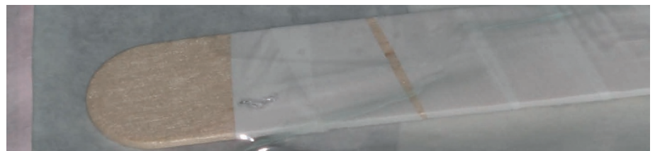
Fig. 2 A strip of PTFE tape supported by a tongue depressor within a sterilisation pouch, after being autoclaved. The PTFE tape remains unchanged due to its high melt viscosity
