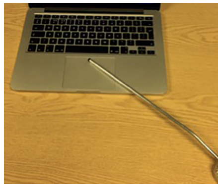
Fig. 17 Addition of a rubber stylus to Patient B's mouth stick
