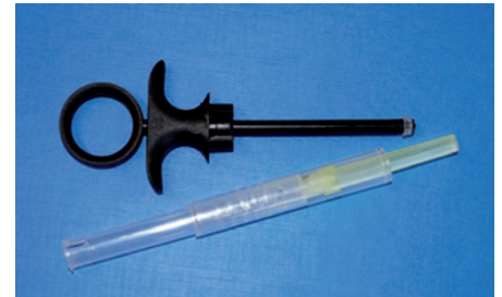
Fig. 2 Example of a 'sharp-safe' syringe design. The outer plastic is drawn down to cover the needle after use. If the outer sleeve is clicked into place once, the sleeve can be retracted again for further use of the syringe. A double click permanently locks the cover into position
