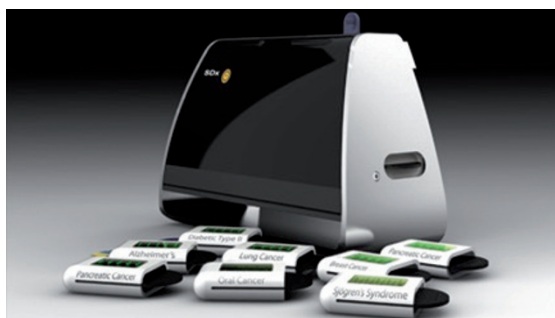
Fig 1 The Oral Fluid NanoSensor Test (OFNASET) technology platform is a point-of-care technology optimized for ultra-sensitive and specific detection of salivary biomarkers for disease detection. In addition it is multiplexable (proteins and nucleic acids RNA/DNA), robust and inexpensive.
