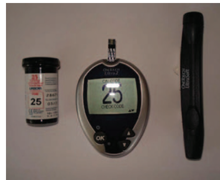
Fig. 1 Blood glucose meter showing coding
