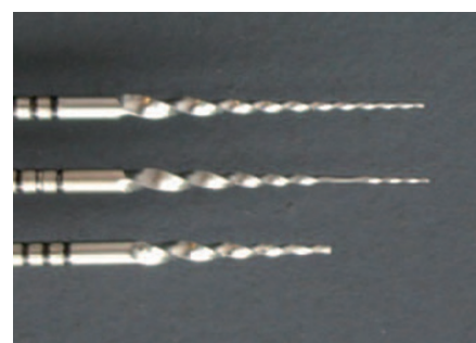
Fig. 3 Three NiTi files showing a brand new file at the top, a file showing evidence of torsional flute damage in the middle, and at the bottom one that has separated
