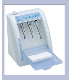
and lubricates up to three instruments at one time, in less than two minutes, ensuring handpiece performance is maintained at all times.
