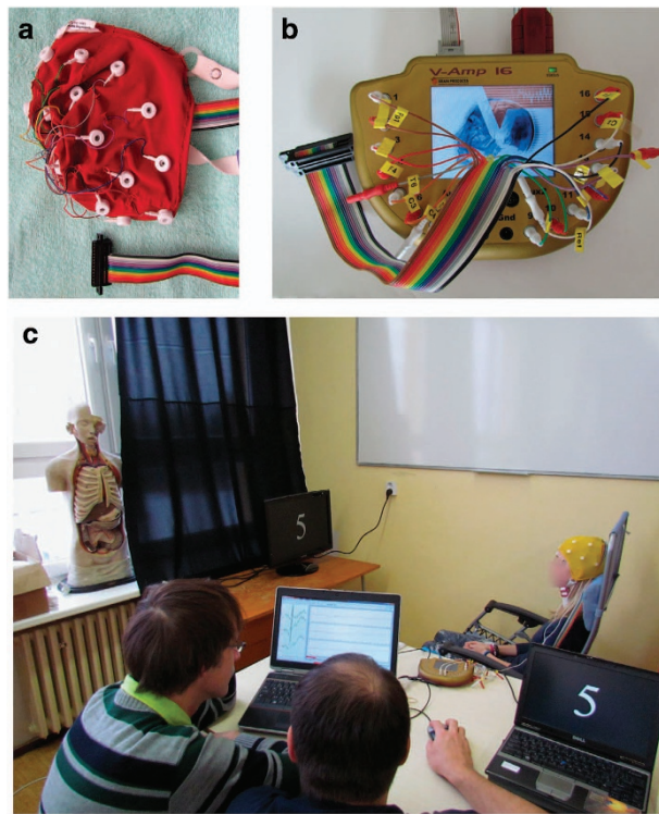
Figure 1. Experiment, hardware equipment. (a) The medium 10/20 EEG cap. (b) The BrainVision V-Amp amplifier. (c) Course of the experiment. Researchers are observing event-related potentials while these are averaged in the BrainVision Recorder. The notebook on the right is used to control the stimulation. The subject sitting in the chair is exposed to visual stimuli. The subject's face has been blurred to protect his/her privacy.
