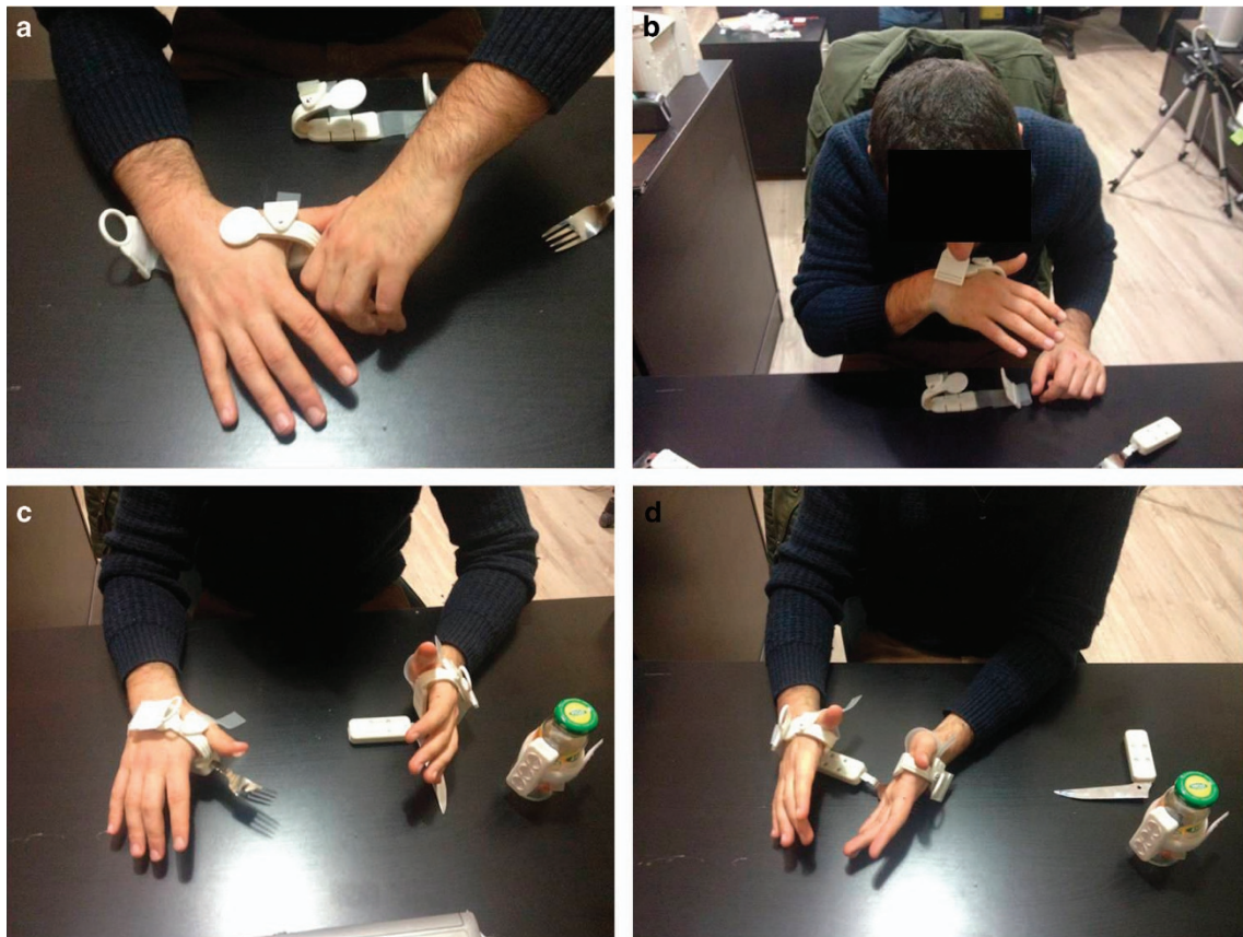
Figure 2. (a) The subject puts his hand into the device; (b) the subject fastens the device pulling the plastic ring with his teeth; (c) the attachment of the 'magnetized' objects; (d) the exertion of a constraint on the objects allows the patient to release the object.
