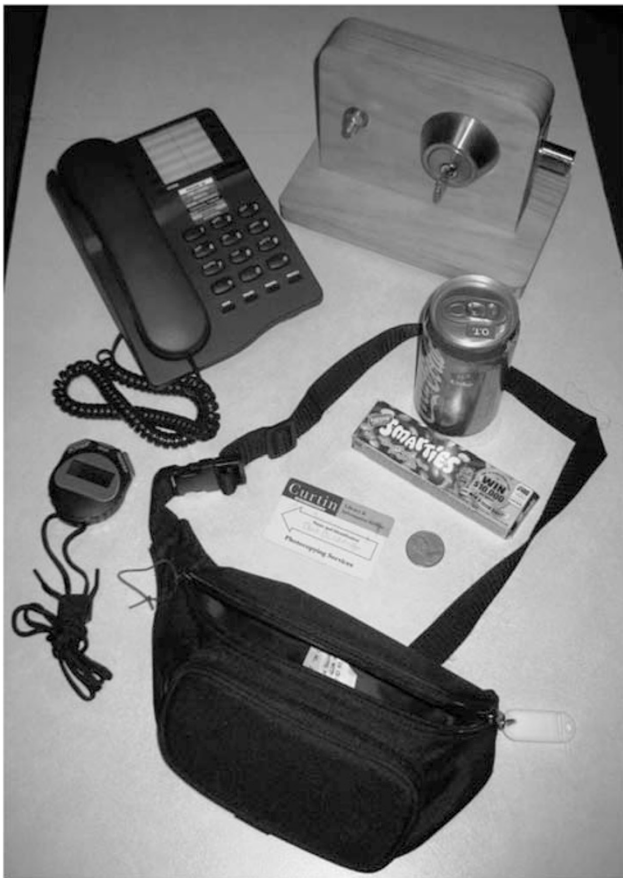
Figure 1 Items of the AuSpinal, including an Australian 20 cent piece coin (diameter = 28.52 mm; thickness = 2.5 mm; weight = 11.3 g), credit card, key, desk telephone, can of drink (375 ml), chocolate-coated candy (1.3 g) and nut (5/8th inch diameter). The stopwatch is used to limit the time spent attempting a task. It is not used to record the time taken to complete a task.
