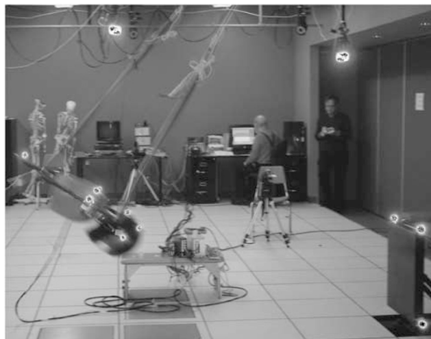
Figure 3 Pendulum method for accelerating the Hybrid III dummy.
