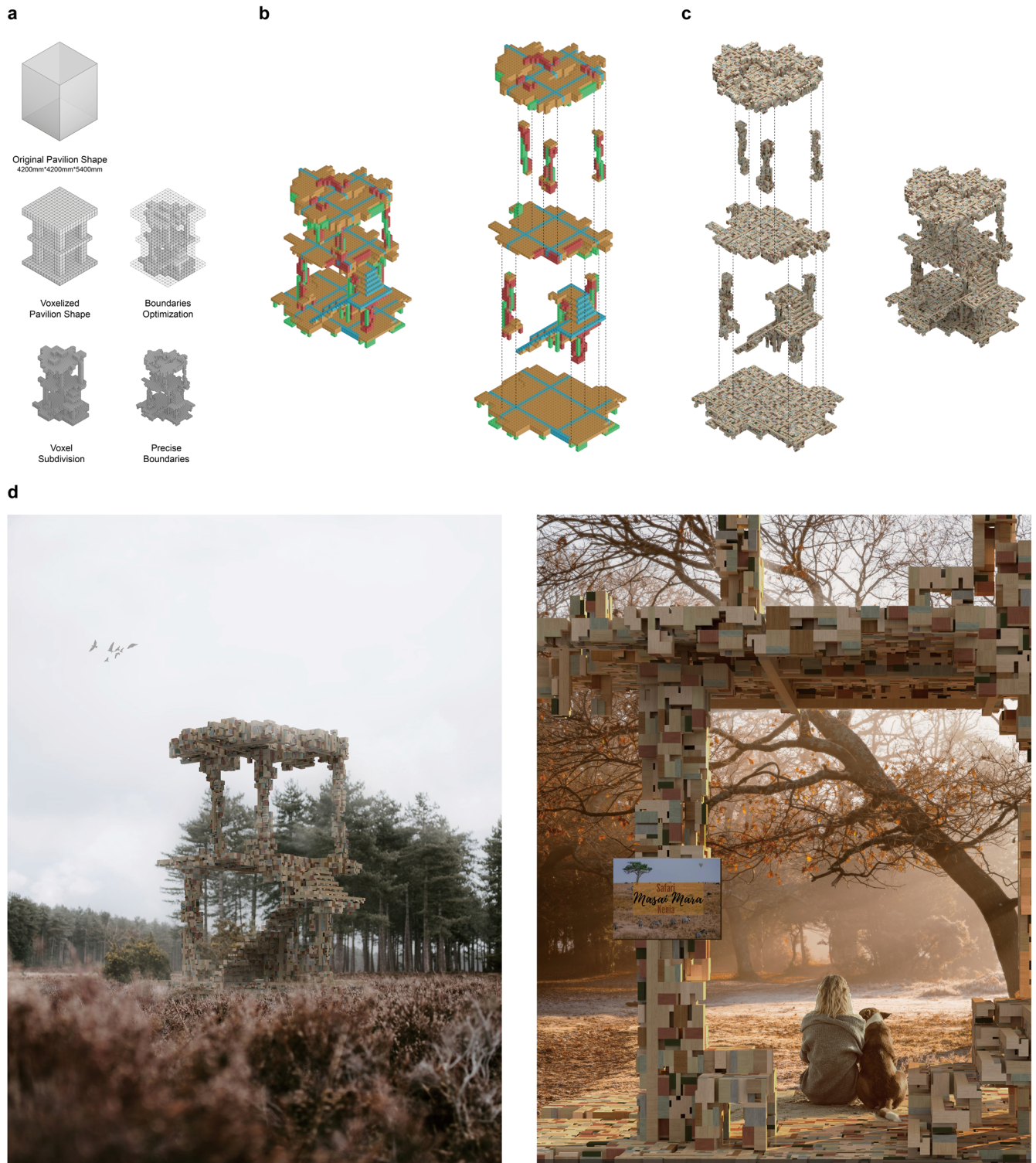
Fig. 6 Sustainable building design proposal and the Primitive Hut. a Voxelized pavilion prototype. b WFC voxel prototype and the exploded-view drawing. c Rendering prototype and the exploded-view drawing. d Two possible environments for the pavilion.
