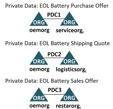
Fig. 10 Blockchain network design for the representative use case. For the representative use case involving an EV OEM, 3 service partners, 3 asset owners, 3 logistics providers, and 3 Re* partners, a blockchain network has been set up using Hyperledger Fabric v2.2 LTS.
