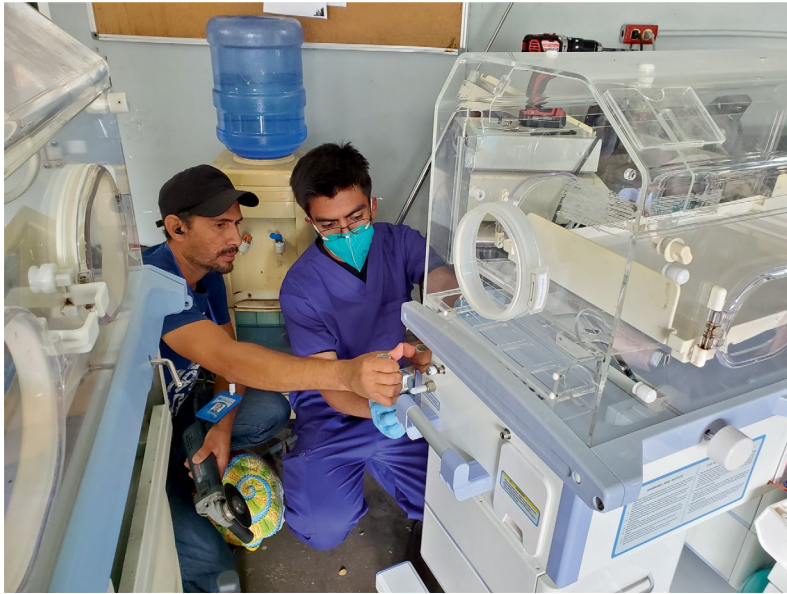
Fig. 1 | Local training as part of the Engineering World Health summer programme. An engineering student works with a local biomedical engineering trainer to repair an infant incubator during Engineering World Health's 2022 Summer Institute in the Dominican Republic.
